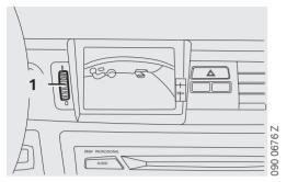
Turn the wheel (1) until the required brightness for the monitor image has been set.
